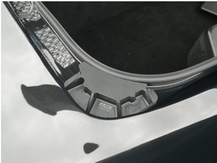
Fig 5: Positioning of the pressure distribution blocks
