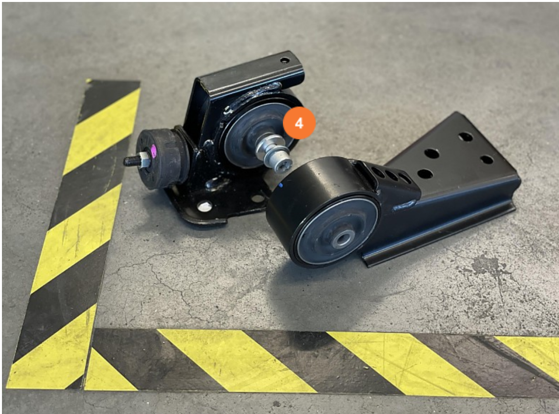
Fig 2: Assembled insulator brackets and insulation washer
