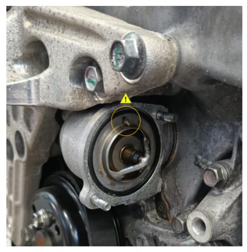
Fig 3: Replacing the thermostat.
