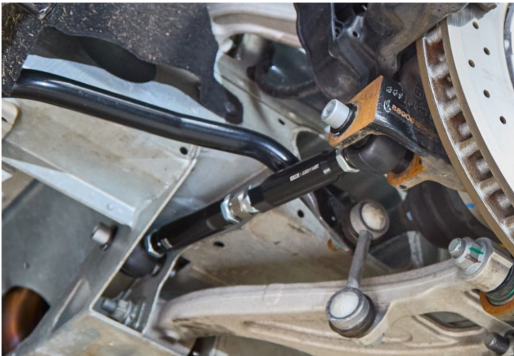
Fig. 5: Assembled upgrade JUBU toe link
