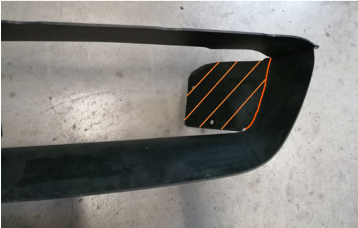
Fig 2: The OEM plastic part has to be trimmed.
