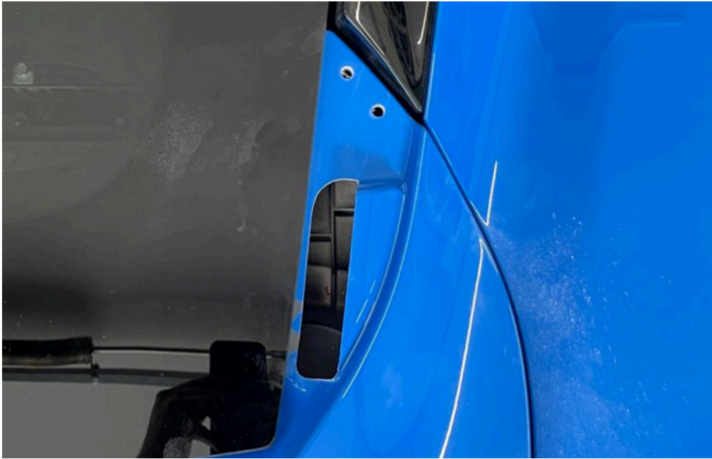
Fig 5: Finished cuts on the top of the engine lid
