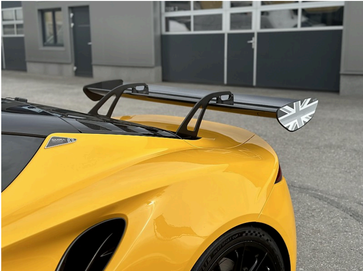
Fig 2: Installed JUBU Carbon swan neck rear wing (Cup EVO)
