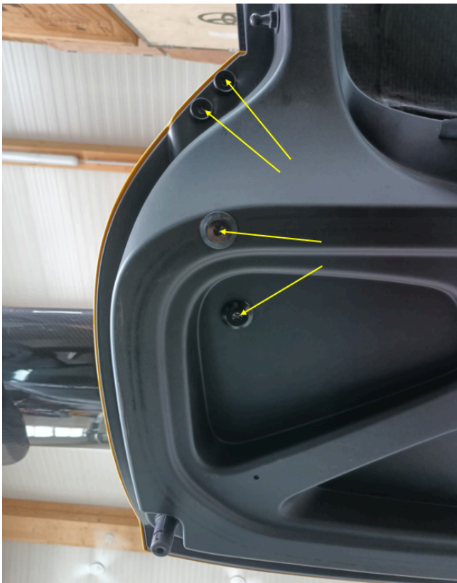
Fig 6: Required holes on the bottom of the engine lid
