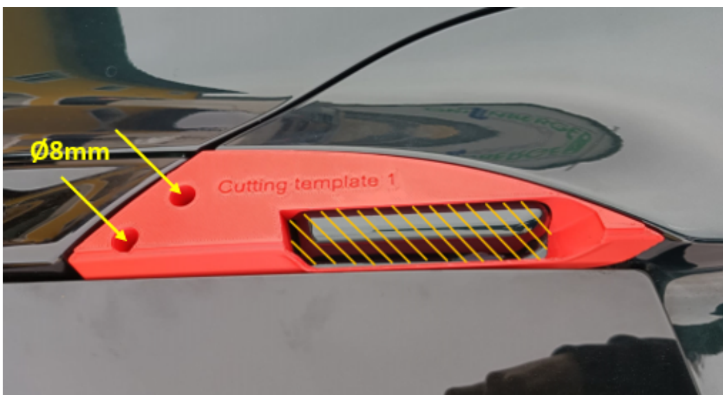
Fig 4: Required cuts on the top of the engine lid
