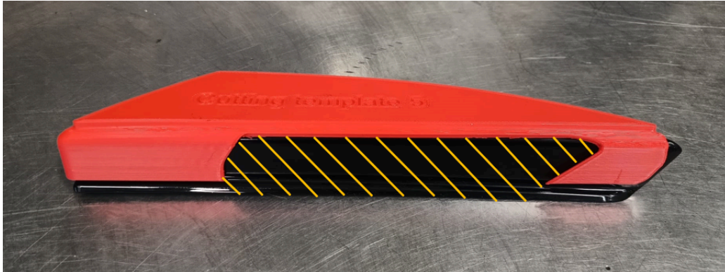
Fig 7: Required trim of the covers next to the rear window
