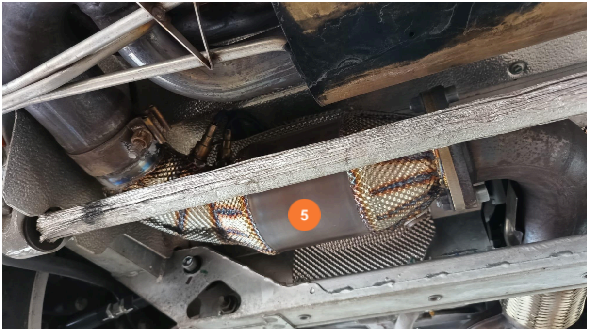
Fig 2: Installing the HD sports CAT-pipe (6)
