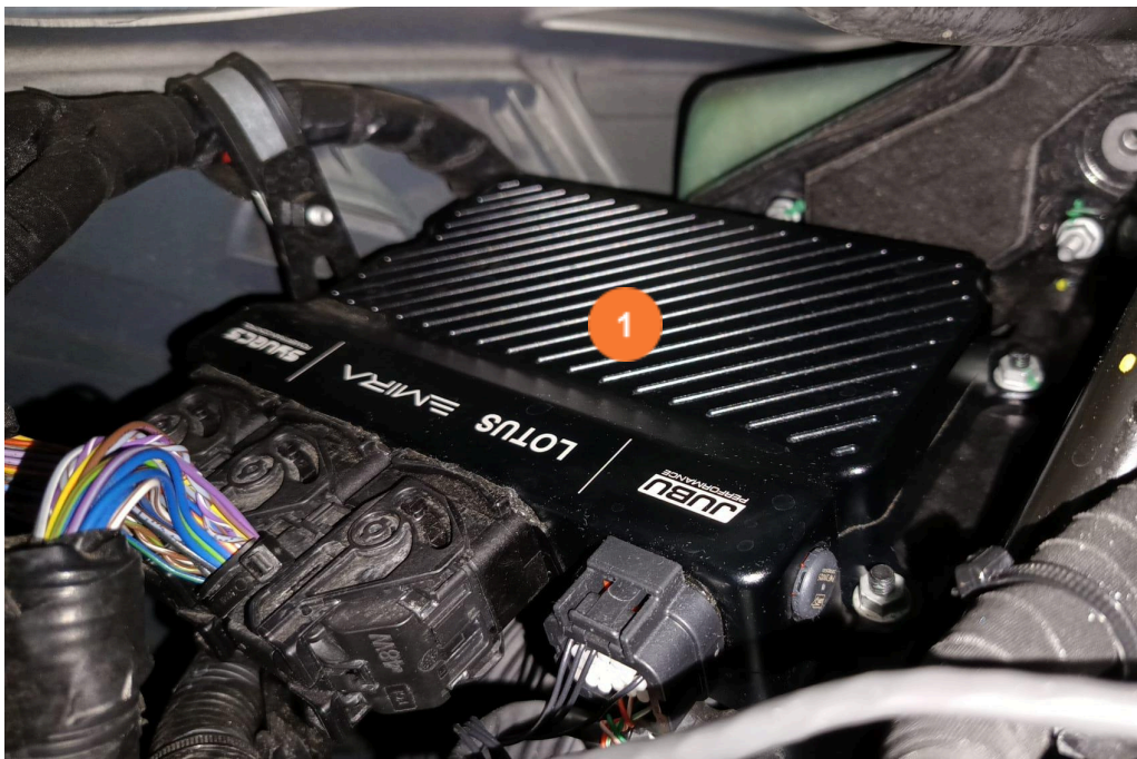
Fig 3: Installing the JUBU Plug & Play ECU Kit (1)
