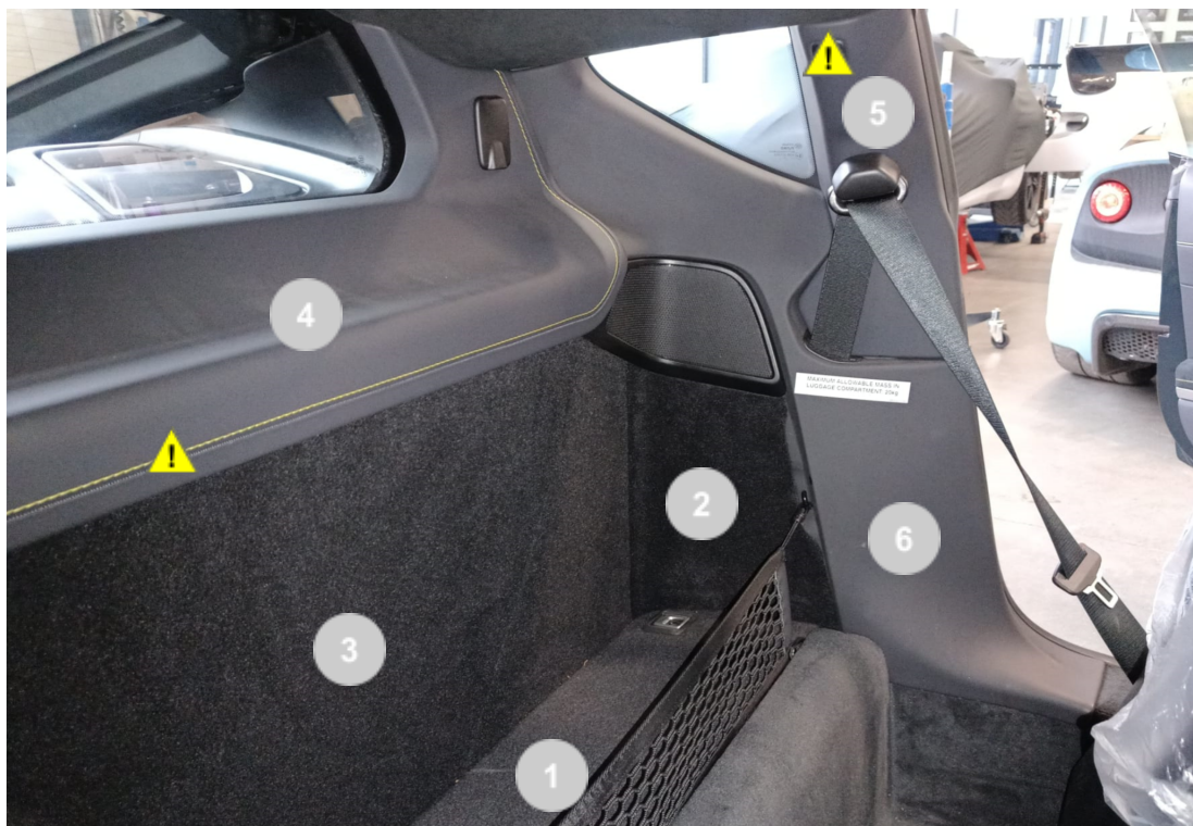
Fig 2: Uninstall the rear interior panels.
