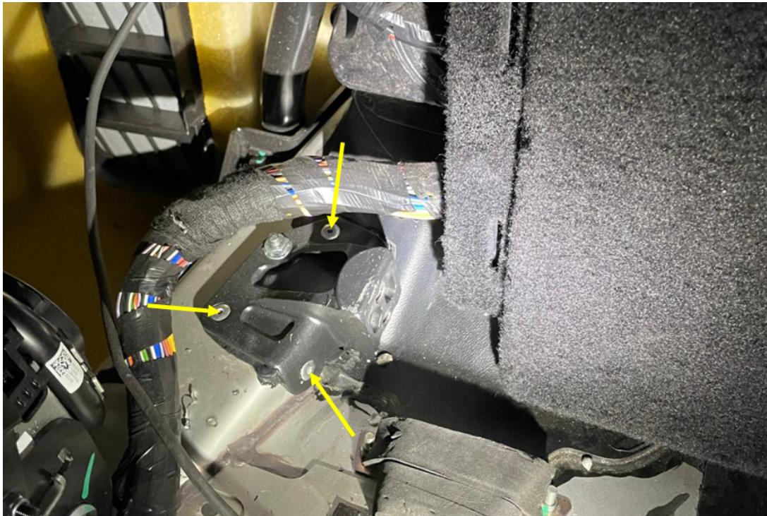
Fig 6: Drill the Ø5mm holes for the right harness bar bracket (4).
