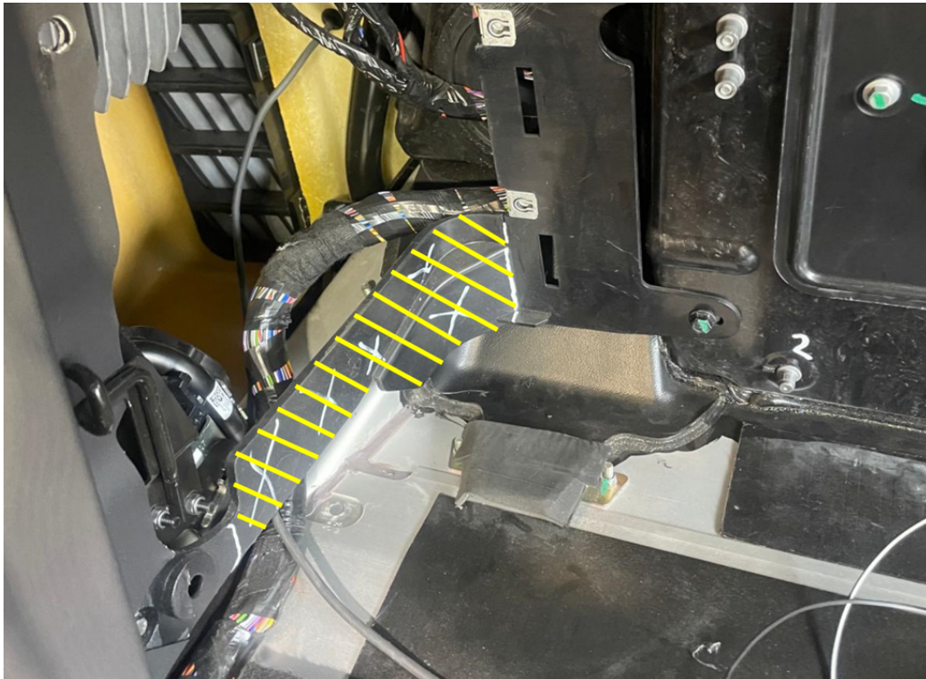
Fig 3: Trimming the plastic brackets in the rear corners.
