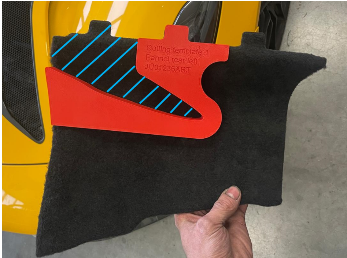
Fig 11: Trimming the panels for the rear corners.
