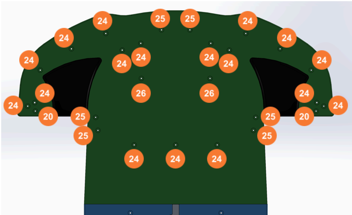
Fig 10: Screw usage on Frontsplitter.
