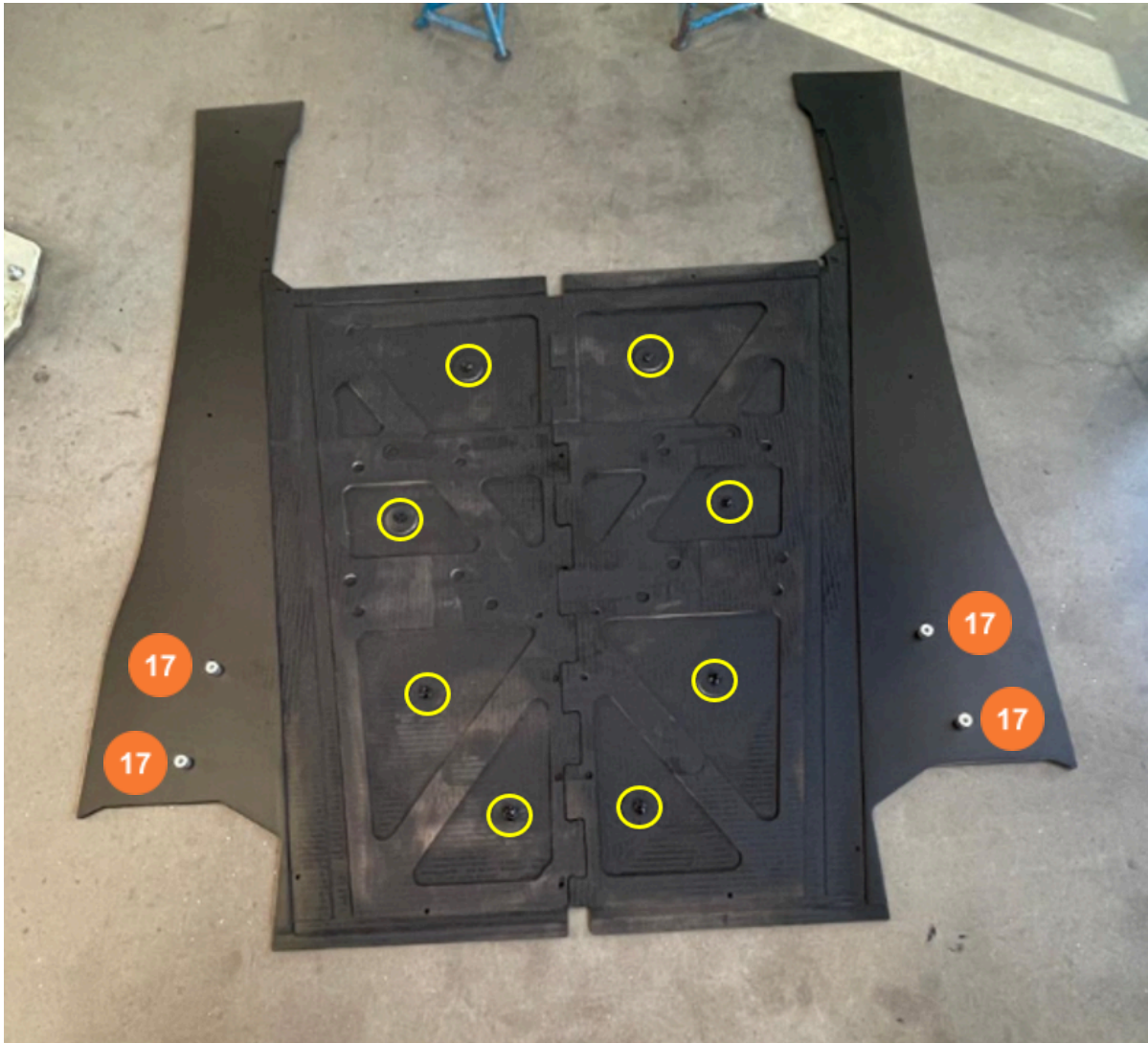
Fig 12: Put bodywork adhesive on the marked areas and prepare the spacers for the A-panels (17).
