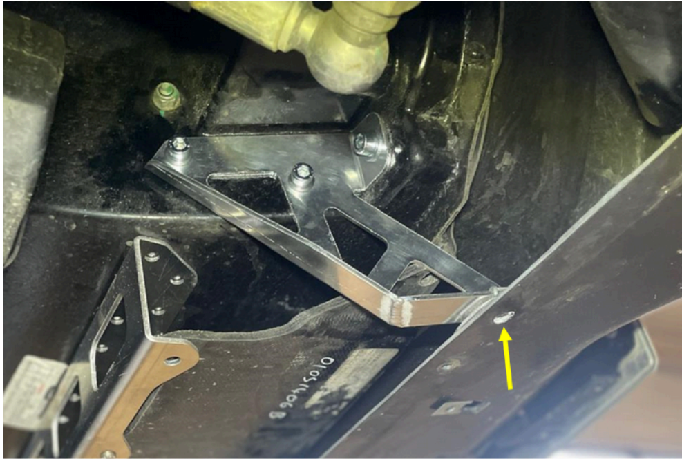
Fig 5: Mounting the frontsplitter bracket (12) and drilling the required Ø7mm into the frontclam.
