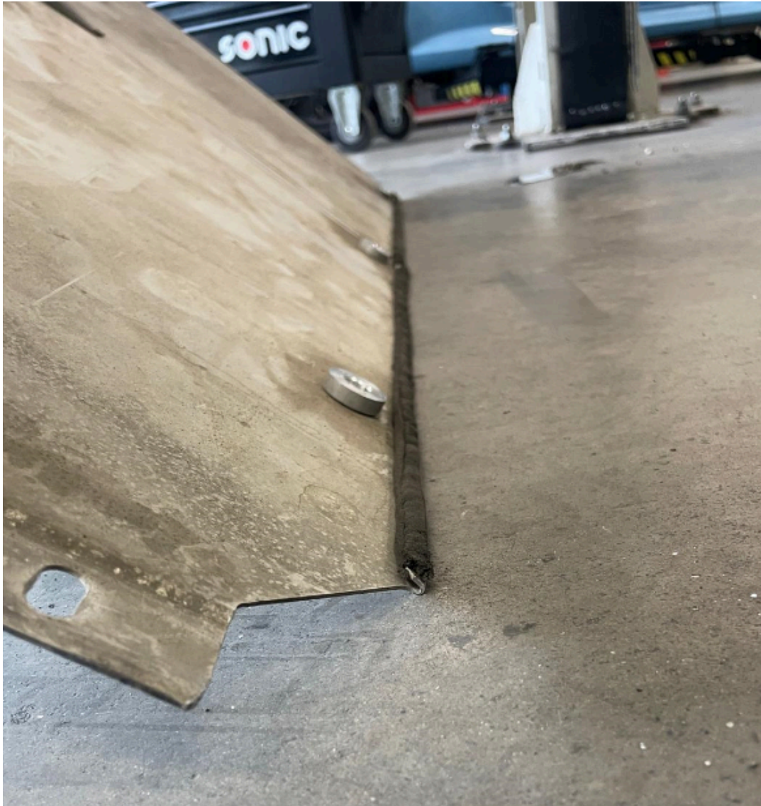
Fig 15: Fold the front edge of the rear undertray plate.
