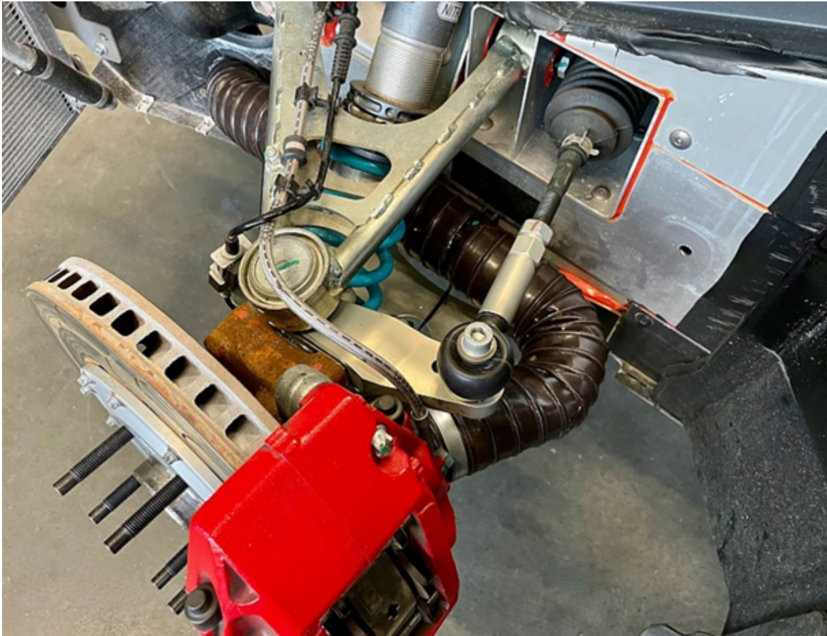
Fig 5: Air Hoses laying (5)
