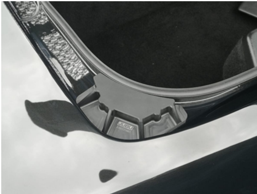
Fig 5: Positioning of the pressure distribution blocks
