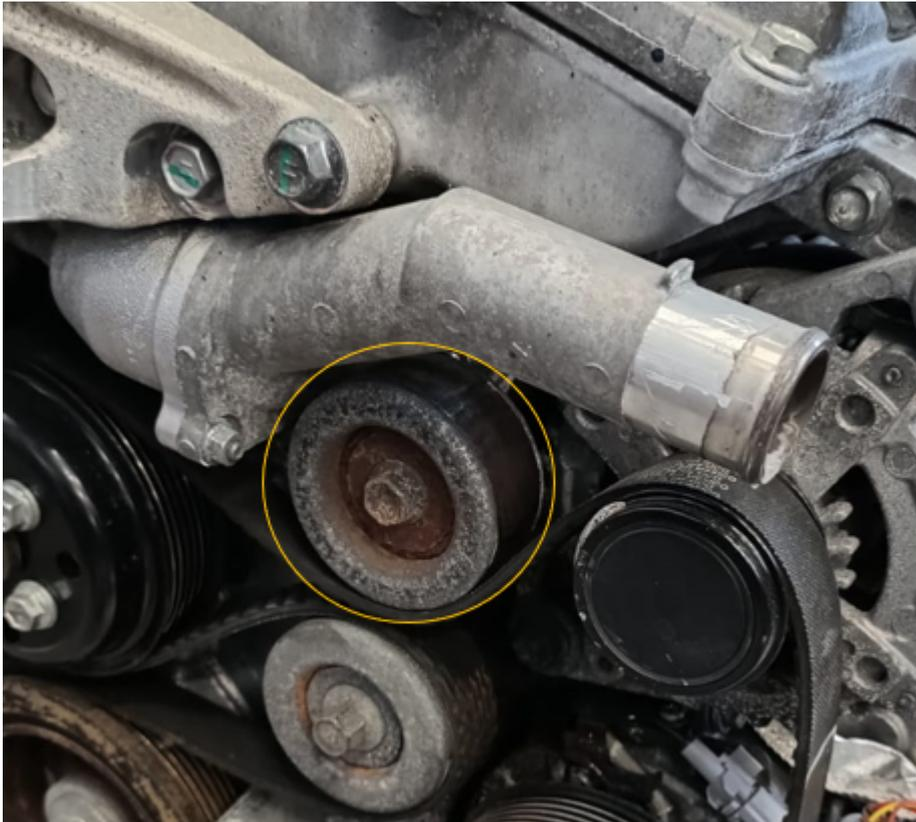
*Fig 2: Remove the pulley next to the thermostat casing.*
