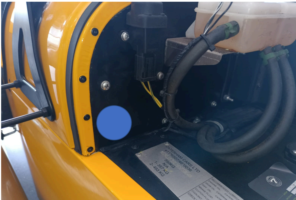
Fig 8: Creating a passage in the bulkhead for the wiring harness (10) on a S3 chassis.
