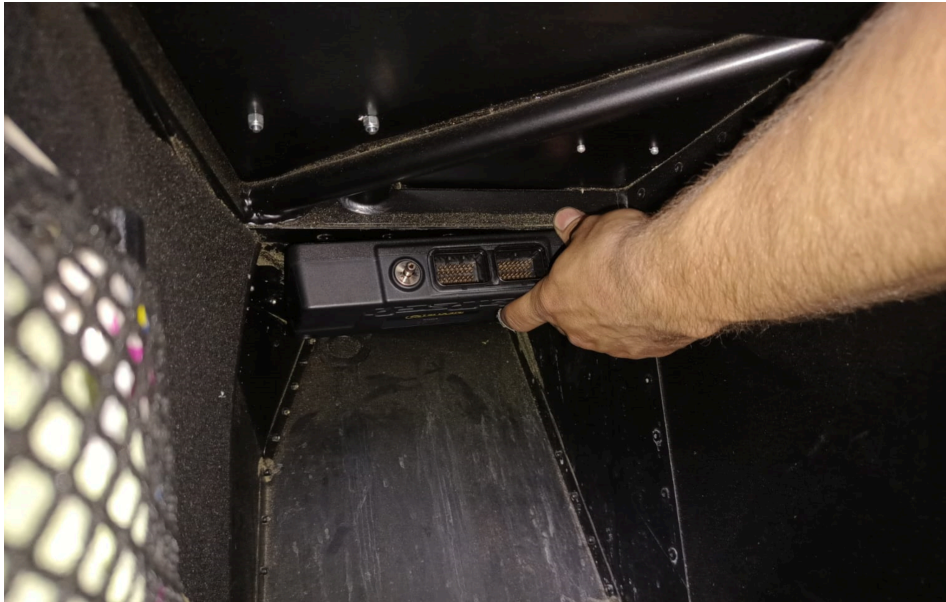
Fig 6: Placement of the ECU (6) in a S3 Chassis.
