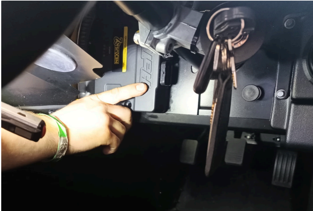
Fig 7: Placement of the ECU (6) in a S5 Chassis.
