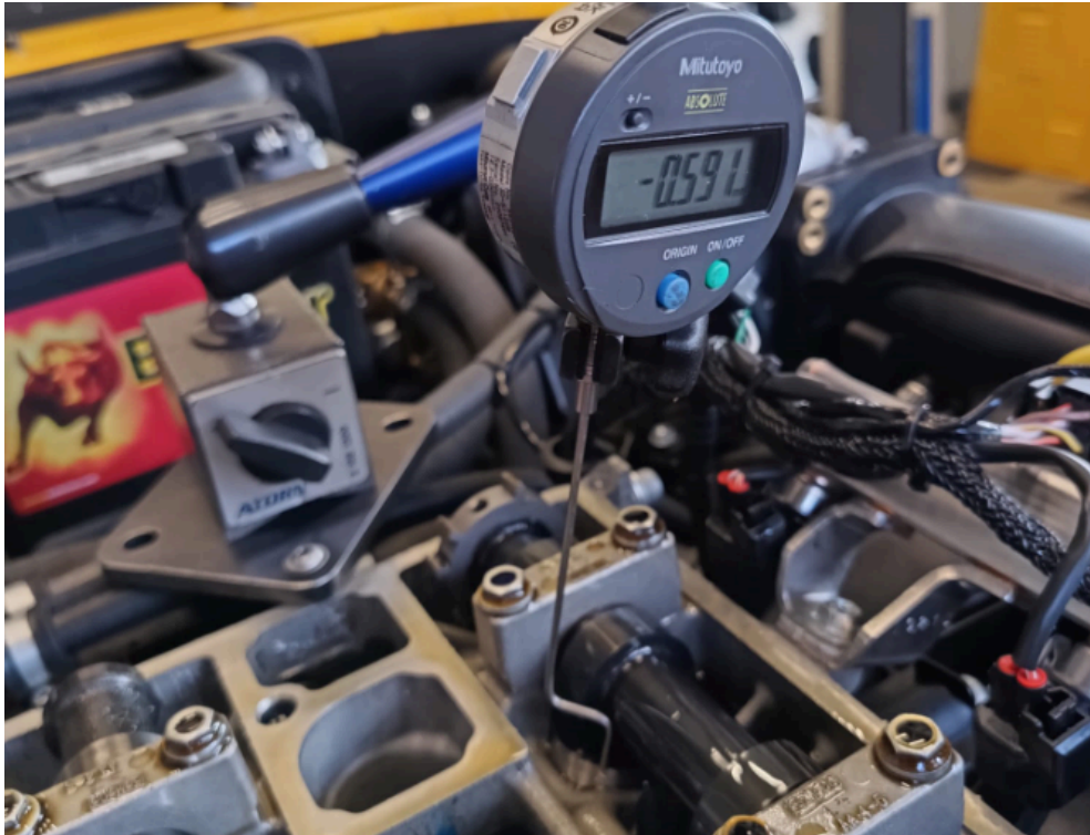
Fig 4: Use a dial gauge to measure the lift on the valve tappets.
